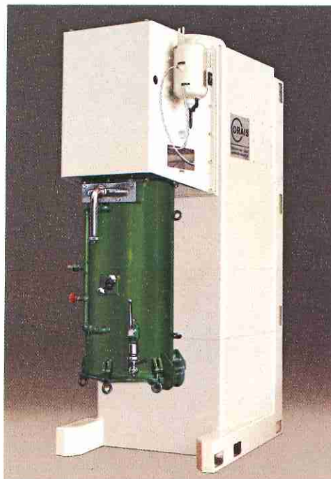
PERL MILL PM 250 TEX of vertical design (above) and with grinding pot of horizontal arrangement (below). ▼
